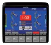
and buzzer if any abnormalities occur. In addition, warning indicators are displayed in four levels to alert the operator of potential issues. Replacement times for required PM services are also indicated.
