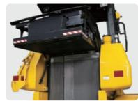
side) radiator, oil cooler and charge air cooler. The hydraulic fan has a cleaning mode which enables the fan to rotate in the reverse direction to help clear off objects that are restricting air flow.
