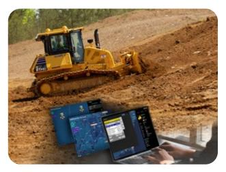
An IMC dozer is capable of dozing to plan with incredible precision and efficiency when working off a 3D design.
