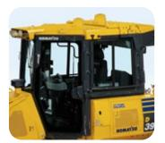
noise and vibration for the operator and discourage dust from entering the cab. In addition, side visibility is enhanced because external ROPS (ISO 3471) structure and posts are not required.
